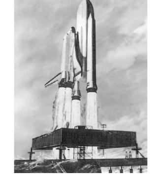
Close inspection of photographs of the take-off assembly will show that the space shuttle and two long, narrow booster rockets are all attached to a very large cylinder in the centre. This large cylinder is not the rocket engine. It is only a storage tank for liquid hydrogen and oxygen, which are fed into the rocket engine of the space shuttle during launch, and then jettisoned.
